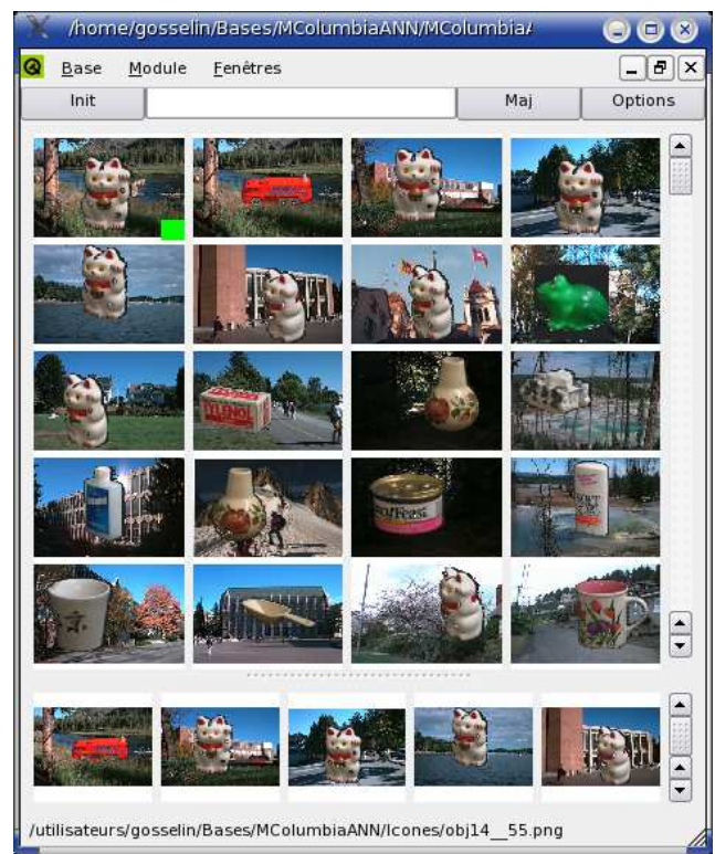
Figure 3: The RETIN graphic user interface. Top part: retrieved images; Bottom part: images selected by the active learner.
