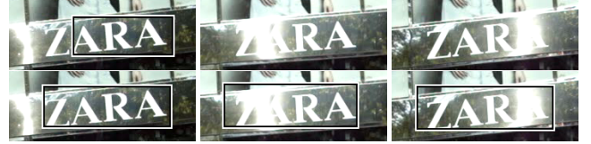
Fig. 2. Top: output of the SnooperText detector to three different frames, showing failures due to illumination changes; Bottom: output of SnooperTrack on the same frames.
