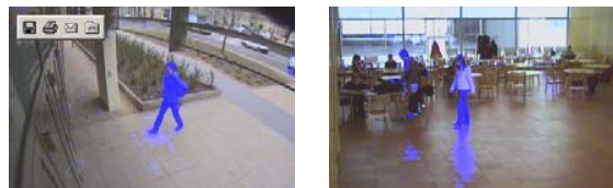
Figure 2: Experimental results: a) a good detection results b) detection problem caused by reflection and shadows
